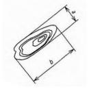
Knot sizes are measured as the average of their largest and smallest diameters
