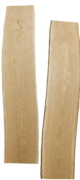
Un-edged oak boules (or selected boards) are appearance graded by means of a virtual grading rectangle measuring 0,20 m x 2 m.
